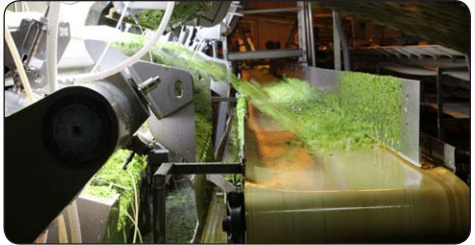
Inside Norpac's Stayton plant, chopped celery whizzes toward a freezing tunnel. Processing vegetables is not just energy intensive: the process also uses plenty of water. Norpac's plants now use 30 percent less water than they did 30 years ago to process their vegetables. That works out to a corporate savings of 450 million gallons per year.
