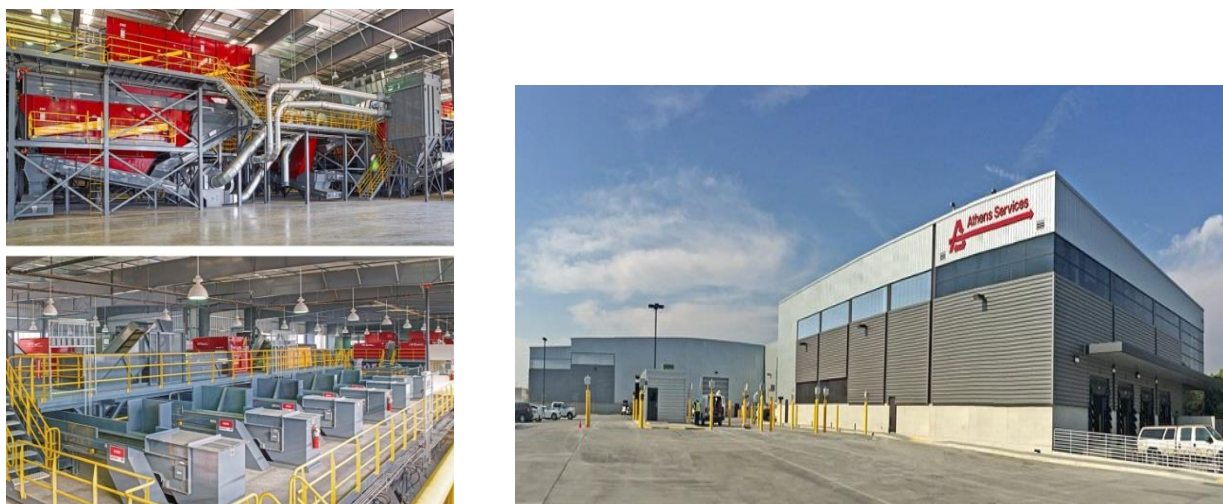
(Pictured above; The Athens mixed waste MRF in Sun Valley, CA Opened in 2014 and processes on average 1,600 tpd)
