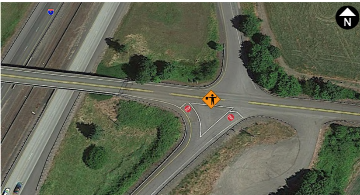
Figure 49. Recommended Ankeny Hill Road/I-5 Northbound Ramps Event Ingress Traffic Control. Note: Traffic control will be provided to monitor ramp queues, no change in traffic control is proposed.
