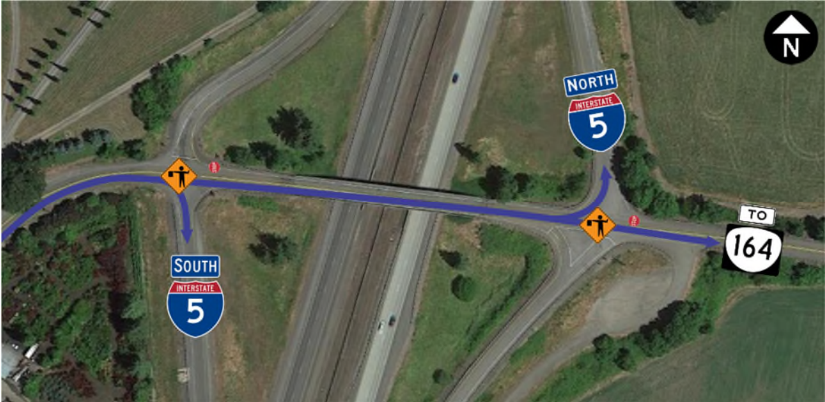
Figure 53. Recommended Ankeny Hill Road/I-5 Interchange Event Egress Traffic Control.
