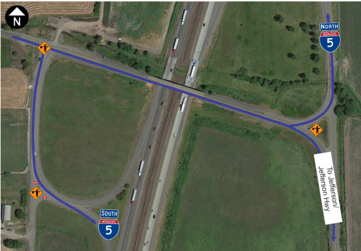
Figure 62. Recommended Talbot Road/I-5 Northbound Ramps Event Egress Traffic Control. Flagging staff will be located with illuminated stations to help manage queues and assist with highlighting the primary routes.
