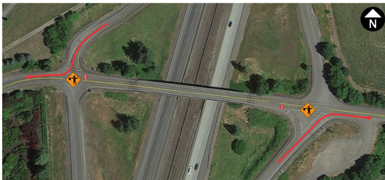
Figure 56. Recommended Ankeny Hill Road/I-5 Ramps Event Ingress Control showing the non-conflicting I-5 Southbound and I-5 Northbound routing. Flagging staff will modify the intersection control and support local access movements while managing and monitoring queues.
