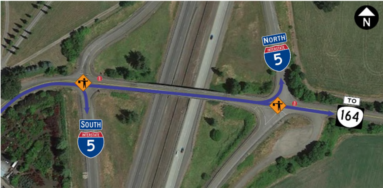
Figure 61. Recommended Ankeny Hill Road/I-5 Interchange Event Egress Traffic Control. Flagging staff will be present with illuminated stations to help manage any queues that form.
