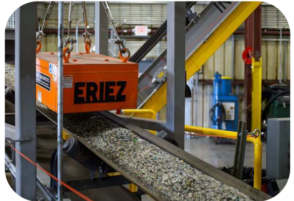
Plastic pellets heading for conversion into oil. Source: www.agilyx.com
