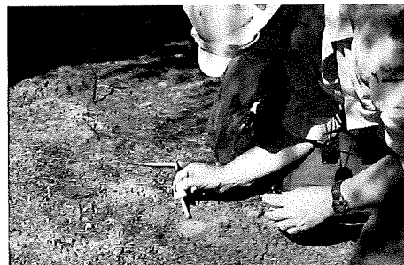
A simple test can determine whether a water repellent layer is present.
