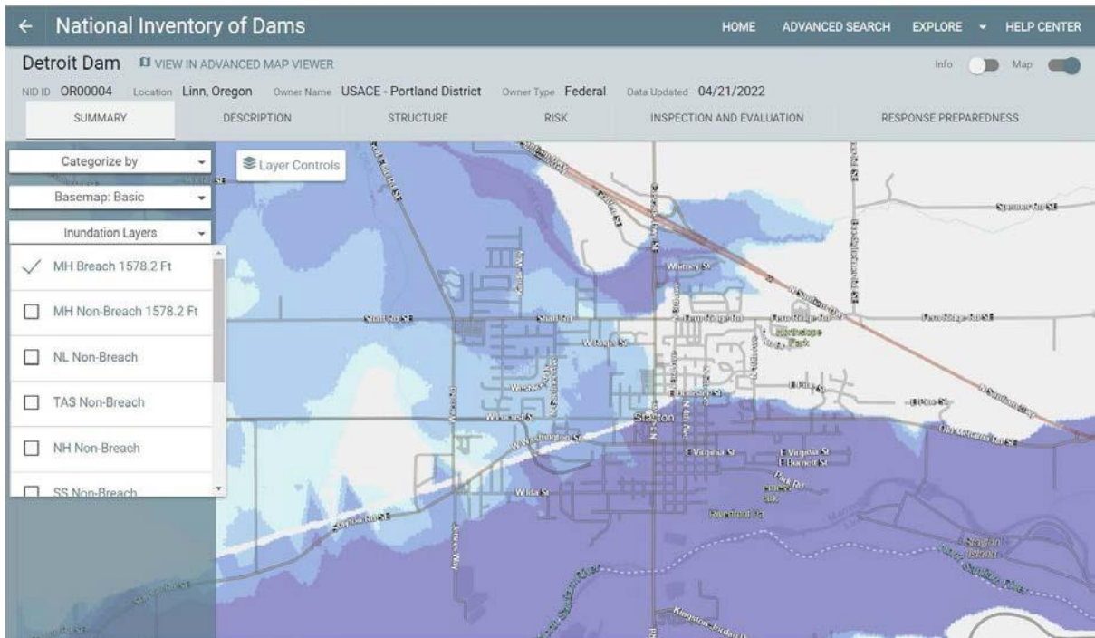
Figure 14-3, Inundation map from the National Inventory of Dams (Maximum Height Breach scenario for Detroit Dam)
